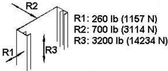
**Figure 2: Support wall configuration**
