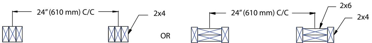
Load bearing wall must be able to support a pull-out force of 700 lb (3114 N) at any point.
