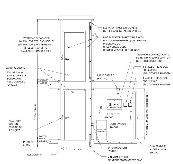
RESIDENTIAL ELEVATORS (REI) CONTROL SYSTEM CONTAINS THE 240 VAC AND 120 VAC DISCONNECTS, HOWEVER; GC/ OWNER MUST PROVIDE DEDICATED CIRCUIT AND WIRE TO 4" x 4" BOX (1 FOR 240 VAC & 1 FOR 120 VAC) IN MACHINE SPACE PER DRAWING. SEE REI ELECTRICAL REQUIREMENTS BROCHURE FOR FURTHER DETAILS.
