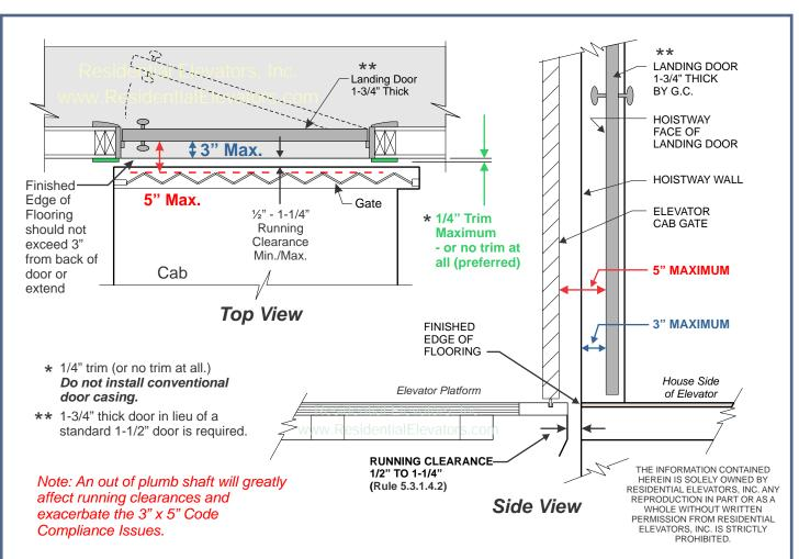
Note: Concrete block / masonry shafts and some commercial metal door frames can often create 3"X 5" Rule violations.
