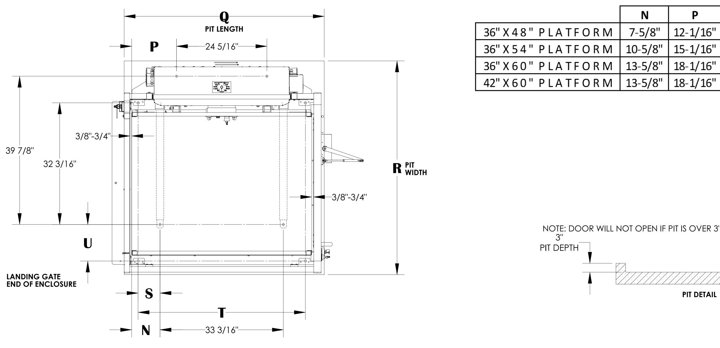
**UNITS WITH STRAIGHT THROUGH PLATFORM WITH ENCLOSURE PIT APPLICATION**
