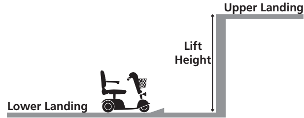
Floor installation = Floor to floor distance
