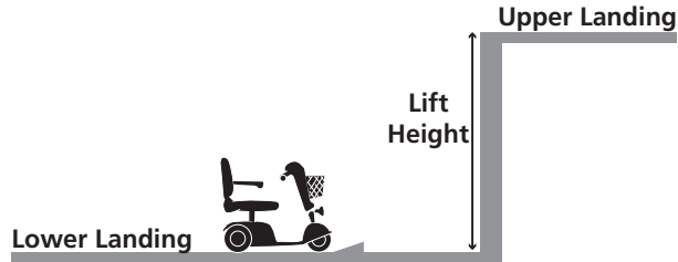
Floor installation = Floor to floor distance
