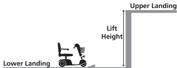
Floor installation = Floor to floor distance
