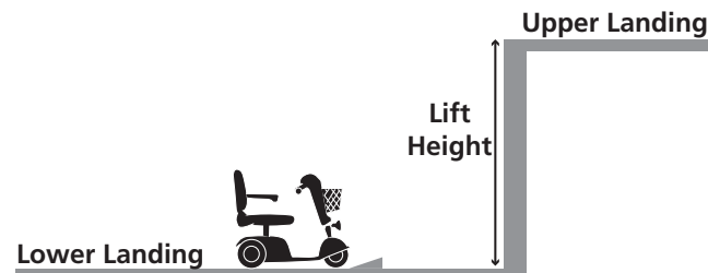
Floor installation = Floor to floor distance
